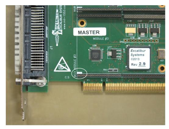
3. Align the Pin 1 marker (marked with a white rectangle) on the module with the white rectangles on the carrier board.
