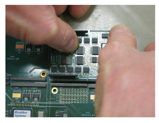
5. Make sure that the module is inserted all the way.
