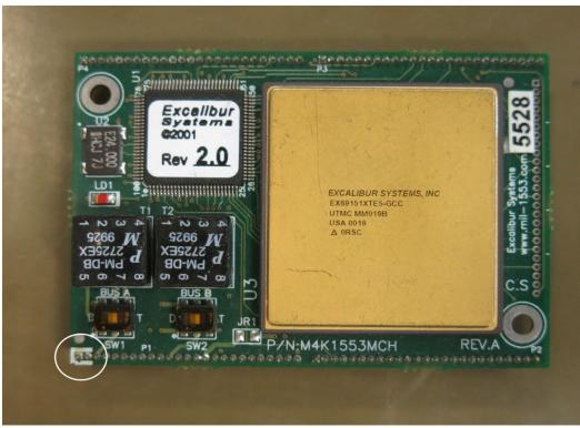
4. Very carefully insert the module into the carrier board.
