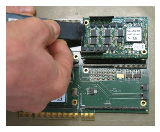
2. Make sure that all the pins on the module are straight, and not bent.
